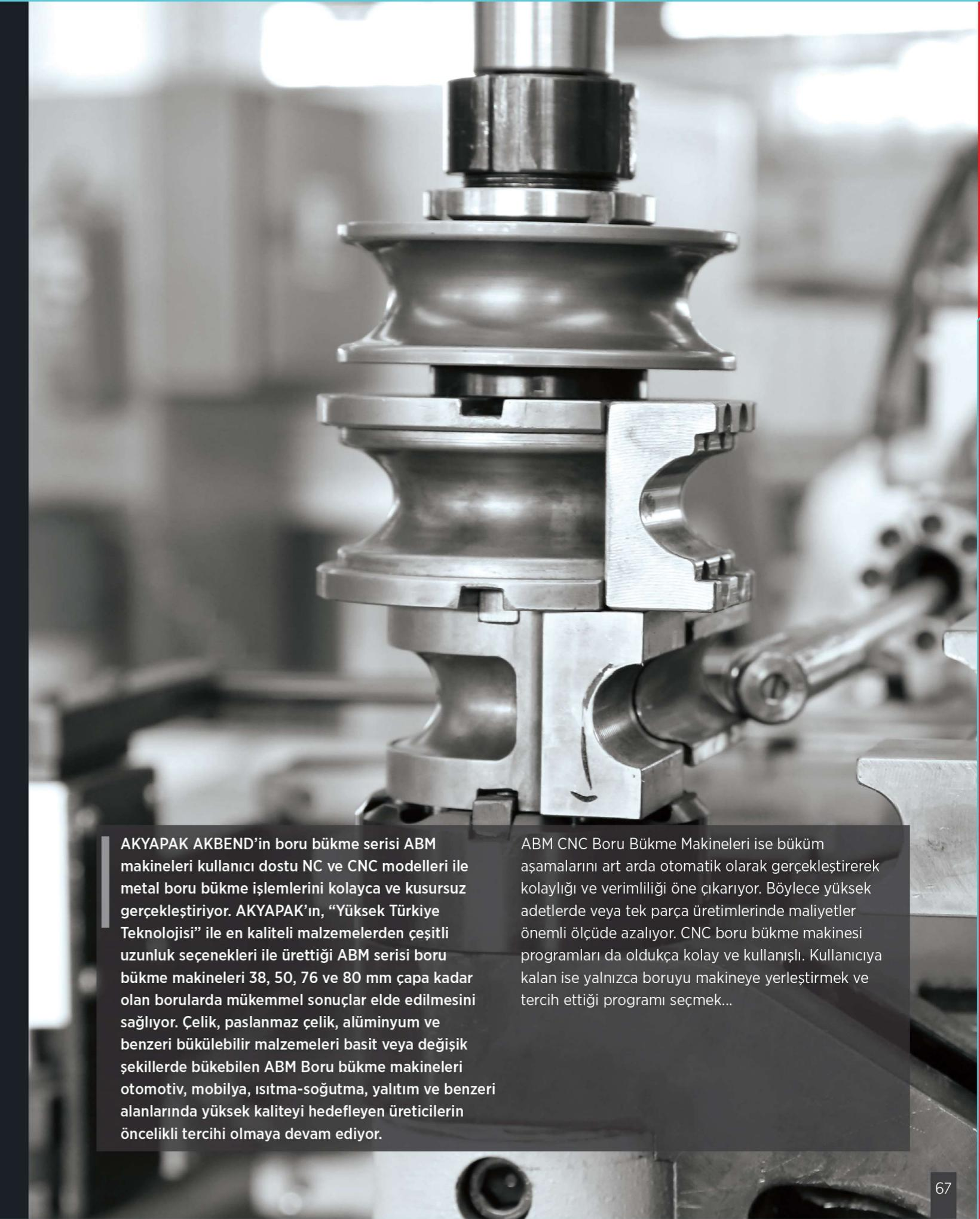
ABM 76 CNC-3 Tube Bending Machine bends tubes up to 76 mm diameter with high quality and accuracy as servo motor controlled. The machine which allows for working with 3 dies provides convenience, prevents waste of time and increases efficiency, through sequential and automatic bending processes via its advanced CNC system.
