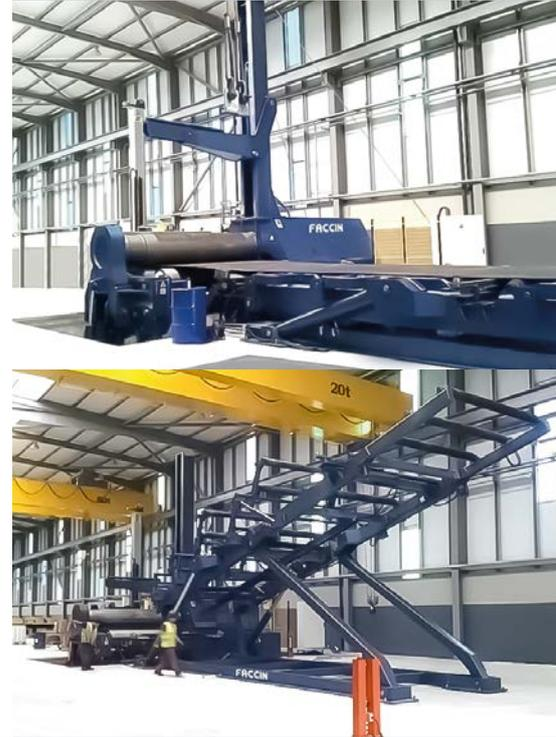
The 4HEP series of 4-roll synchronised bending rolls is the latest design evolution developed by Faccin and tested by the most demanding operators in extreme environments for over 25 years. It combines power, reliability, and precision in an exclusive package, making it the state of the art in modern plate rolls.
