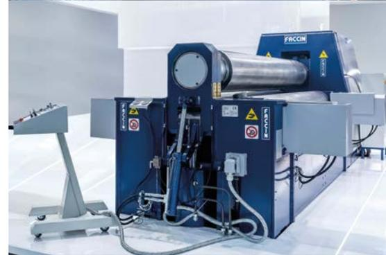
Thanks to the horizontal position of the cylinders for lower roll movement, HAV 3-roll variable axis bending rolls are equipped with a reduced height work top. No foundations are therefore required, even for bending rolls with capacity up to 40 mm.
